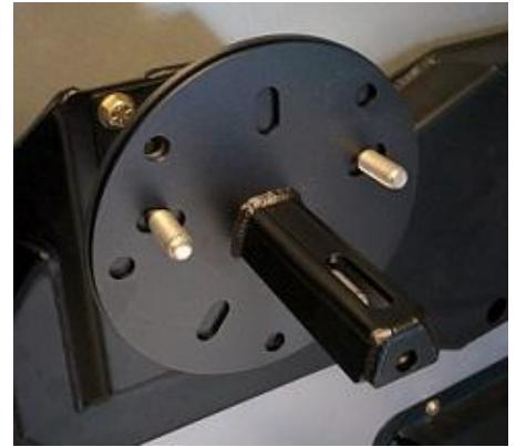
2. Install the spare tire, sandwiching the stud plate between the tire and tire carrier. Tighten the lug nuts to the studs.
