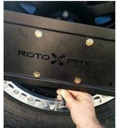
7. To install for use as a license plate relocate and not a gas can mount, thread the supplied ¾" long bolt locknut and washers through the slot in the center. Slide the bracket to the desired depth and tighten the bolt, clamping the sliders together.
